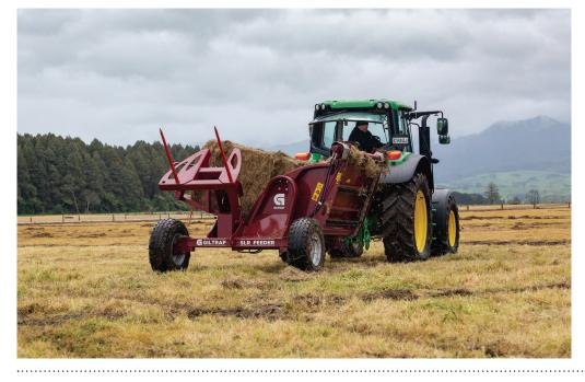
also has a reinforced frame and extra-large tandem axle and tyres.
