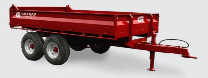
All Giltrap trailers are designed to tip to at least 55° to fully unload, even with wet or sticky products.
