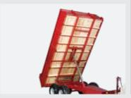
The sides and front are fabricated from 3mm steel plate for strength and rigidity. Sides are hinged so they can be quickly dropped or removed. Giltrap's simple locking system makes this easy.
