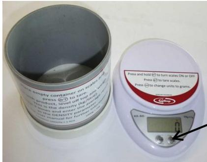
Turn scale on by pressing and holding button marked  $\phi/T$
