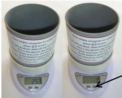
Place empty cup on scale and then zero scale by pressing button marked  $\phi/T$
