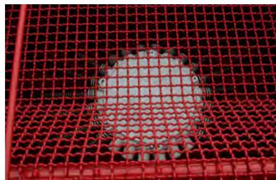
Mesh screen and distributor head in the hopper
