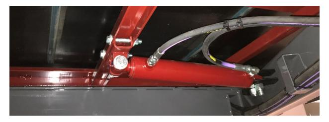
To operate, connect the two side shift hydraulic hoses to the tractor and adjust cross conveyor position using the tractor hydraulics.
